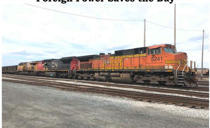
Foreign power continues to flow in and out of Curtis Bay Yard in Baltimore. Seen here are three such locomotives from various lines to the north and west. In the lead is BNSF 5241, a GE C44-9W built in April 2002, followed by CN 2136, a GE C40-8W built in April 1992 as ATSF 802. In third place is UP 7994, a GE AC45CCTE built in June 2012 as an ES44AC.
